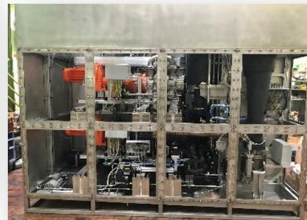
Serial testing of diffusion and ring pumps.
