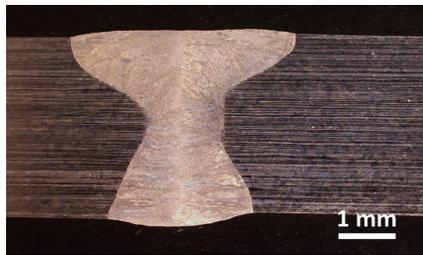
*In-bore laser weld sample*
