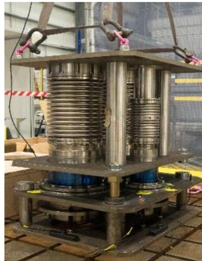
*Pipe alignment testing*
