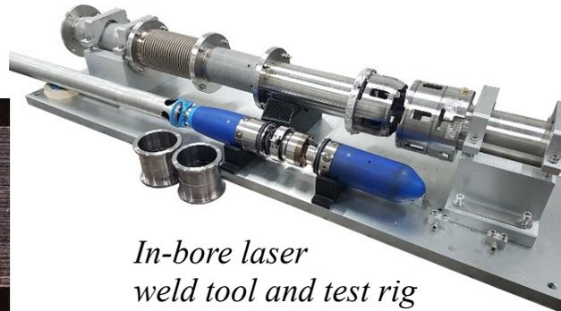
*In-bore laser weld tool and test rig*
