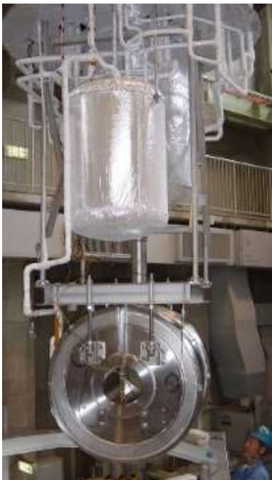
R&D coils for subcooled tests using NbTi/Cu/Al conductors for LHD helical coils (2002-2005)
