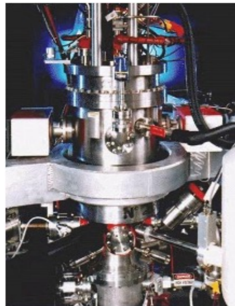
NIST-EBIT (米国) E_e < 33\text{keV} , I_e = 150\text{mA}
