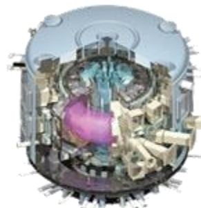
ITER 800 m 3 (one-third the size of an Olympic swimming pool) ~ 500 MW th
